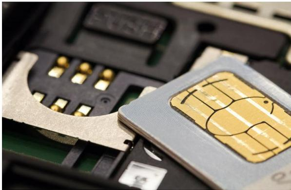
Secure Elements (SE) are a chip-based solution for mobile payment that enables secure storage of payment transactions and other sensitive credentials. Secure Elements in any of their form factors USIM cards (UICC), Embedded SE (eSE), SD cards or add-ons are one of the most secure and reliable solutions for NFC payments market.
